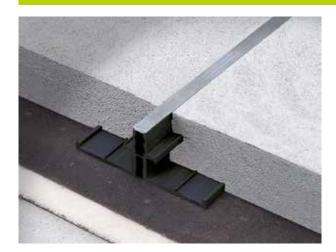
Joint recommended for mortar laying, manufactured from double-density synthetic material. It is composed of two rigid structural parts joined by soft plastic coated material inserts, available in multiple colors. The CMB joint is used to split the subfloor or screed as required by the project.
